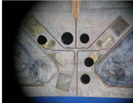
Figure 1: A 660 GHz sideband separating mixer fabricated by Dr. Groppi for the Space Research Organization of the Netherlands. Critical dimensions are controlled to  $\pm 2.5\mu\text{m}$
