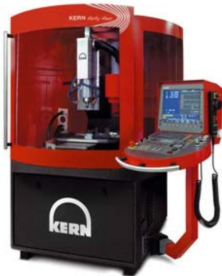
Figure 2: The Kern Model 44 micromilling system used in ASU's SESE THz laboratory.
